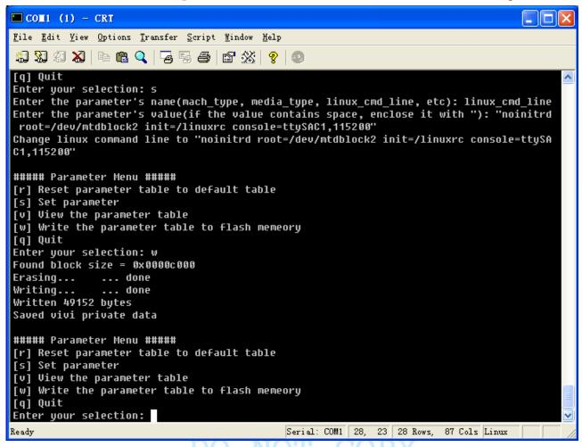
Now when the system reboots, the booting and login messages will be output at serial port 1 and vivi's messages will still be output at serial port 0.
