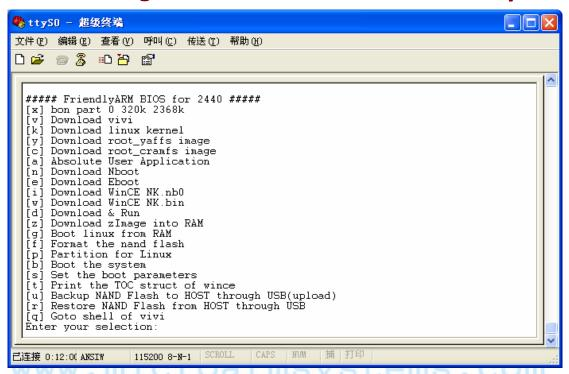
SUPERVIVI is developed and maintained by Friendly Arm, it is based on vivi. It starts with a function menu. And users can switch between supervivi's menu interface and command line.
