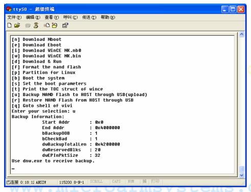
(3) Start the DNW application. Connect the board to the PC via a USB cable. If the DNW's title bar shows "USB:OK", it indicates the USB connection is a success. Go to "USB Port" -> "Backup NandFlash to File"
