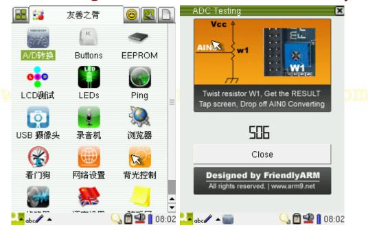
Turning the W1 adjustable resistor, you will see the conversion changes. It has 10 digit precision, therefore the minimum value is close to 0 and the maximum value is close to 1024.
