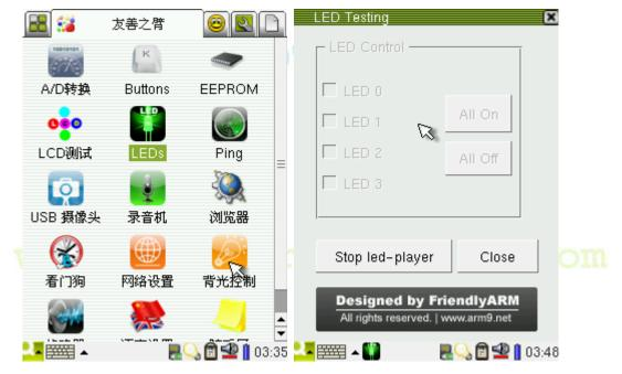
On the popup window, the "Stop led-player" is enabled. This is because the led-player service is started on system startup. After the system boots up, you will see a "sequential led lighting" which is played by this service. To control a single LED, close this service to release the LED resources.
