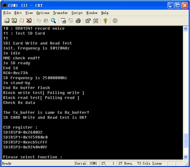
These messages show that SD card access is successful. After the test is done it will automatically return to the main menu.
