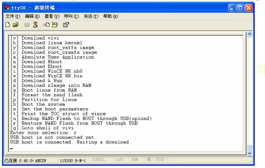
(3) Start the DNW application, connect the board to the host PC via a USB cable. If the DNW's title bar shows "USB:OK", it indicates the USB connection is a success. Go to "USB Port" -> "Transmit/Restore"
