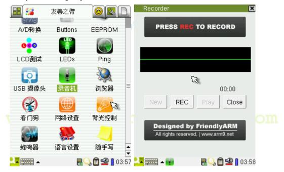
Click on the "REC" button to start recording. When you speak to the microphone on the board, you will see audio waves shown on the screen. Click on the "STOP" button to stop recording.
