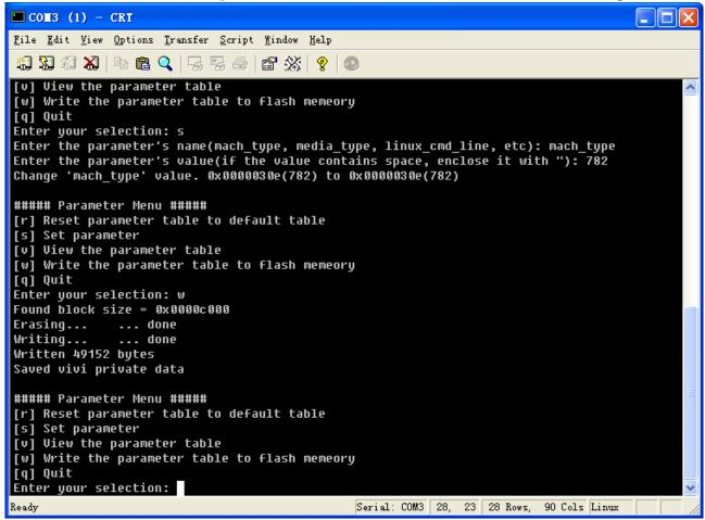
Linux\_cmd\_line is another very important parameter, for example, to change the kernel boot information and change the login port to serial port 1 (the default serial port is 0), you can do it this way:
