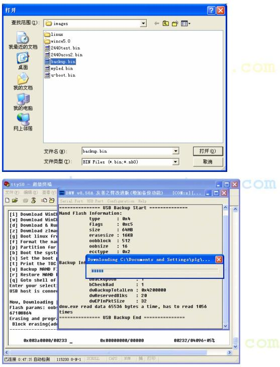
After the process is done, switch the boot mode to the Nand Flash side, and reset or power on the board.
