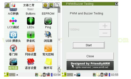
By default, the output frequency of PWM is 1000Hz. Click on the "Start" button, the buzzer will beep. Clicking on the "+" or "-" button will change its frequency and sound as well. Clicking on the "Stop" button stops the buzzer.
