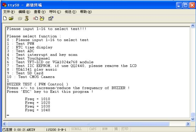
Press the "-" key, the buzzer's frequency will decrease, press the "+" key; the frequency will increase; press the "ESC" key, you will exit the test and return to the main menu.
